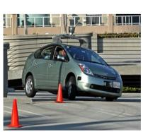
e Google driverless car is powered by artificial intelligence that utilizes the input from the video cameras inside the car, a sensor on the vehicle's top, and some radar and position sensors attached to different positions of the car. Sounds like a lot of effort to mimic the human intelligence in a car, but so far the system has successfully driven 1609 kilometers without human commands.
