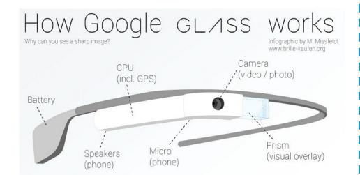
oogle Glass is an optical head-mounted display designed in the shape of a pair of eyeglasses. It was developed by X (previously Google X) with the mission of producing a computer. Google Glass displayed information in a smartphone-like hands-free format. Wearers communicated with the Internet via natural language voice commands.
